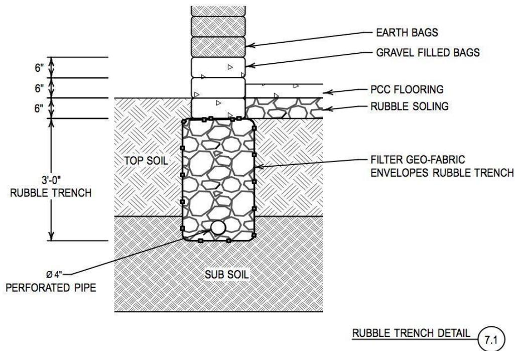
**Figure 2:** Rubble Trench Foundation
