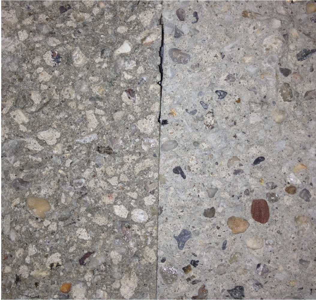
Figure 8: Tensile fracture plane of .8 w/c ratio specimen made with RCA; the sample on the left had a RCA w/c ratio of about .6, whereas the sample on the right had a RCA w/c ratio of .8
