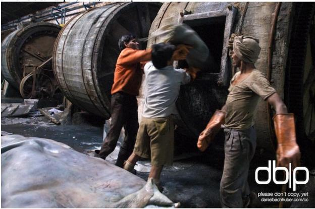
Workers at one of Kanpur's four hundred tanneries, the city's primary industry, load hides into well-used tumblers. Treating leather in this manner is a multi-step process requiring chemicals such as chronium and copious amounts of water. After the water is used, rendered highly polluted in the process, it is genenrally piped back to the Ganges without any treatment.
