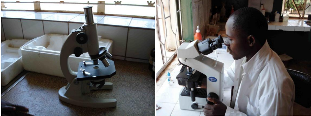
Figure 6: Monocular microscope (best suited to a 6 th form Biology class – not powerful enough to carry out necessary analyses)
