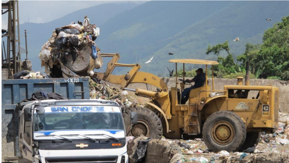
Figure 5: Truck at a garbage transference plant called “Julian Blanco,” where larger containers are filled to take garbage to the landfill.
