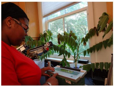
Image 3. Photosynthetic measurements were made using the Licor<sup>®</sup> 6400.
