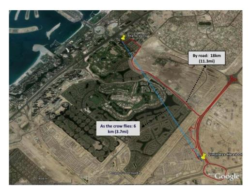
Figure 3: The lack of places to turn left tripled the distance of my evening commute home. The morning commute was 1/3 as long, because of more opportunities to turn right. With a grid many times coarser than Manhattan, everyone lives, works and shops on large islands surrounded by a ring of asphalt and sea of sand. Although this Google photo depicts a largely low-rise area, there are in fact a number of 40-70 story buildings along the Gulf's edge in Dubai Marina.
