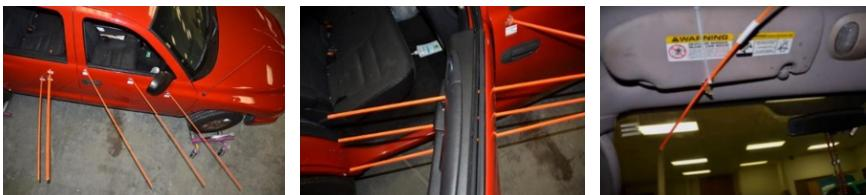
Figure 12: Projectile trajectory markers.
