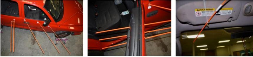
Figure 12: Projectile trajectory markers.
