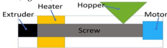
Figure 2. Diagram of a filament extruder.
