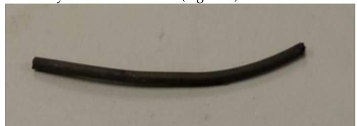
Figure 3. Conductive graphite filament sample.
