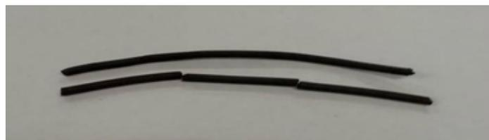
**Figure 4.** A picture comparing the length of two conductive graphite filament samples. Visual confirmation shows that they are similar in size. Note: The bottom piece was broken after having the mass and resistance measured. The top piece is sample 10. The bottom one is 8.
