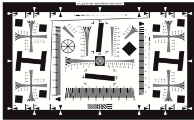
Figure 5: Resolution test chart
